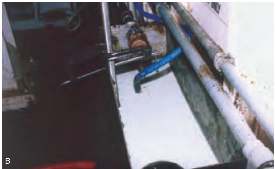
Fig. 1—Emulsifiers in oil-based lubricant can become unstable as they dilute among tramp oils, allowing segregation of lube ingredients such as fats, resins and base oils. This is shown as buildup on a press-lubricant-applicator reservoir (A). Some synthetic lubricants not only do not build up, they can remove previous buildup, as shown on a similar reservoir (B).
