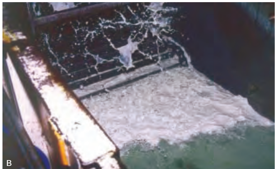
Fig. 2—This photo of a blank-wash reservoir shows how tramp oils remain in the emulsion of an oil-based lubricant (A), complicating recycling operations. A photo of the same reservoir with synthetic lubricant (B) shows how green prelude contamination floats rather than emulsifying into the bath, making contamination removal a more simple process.
