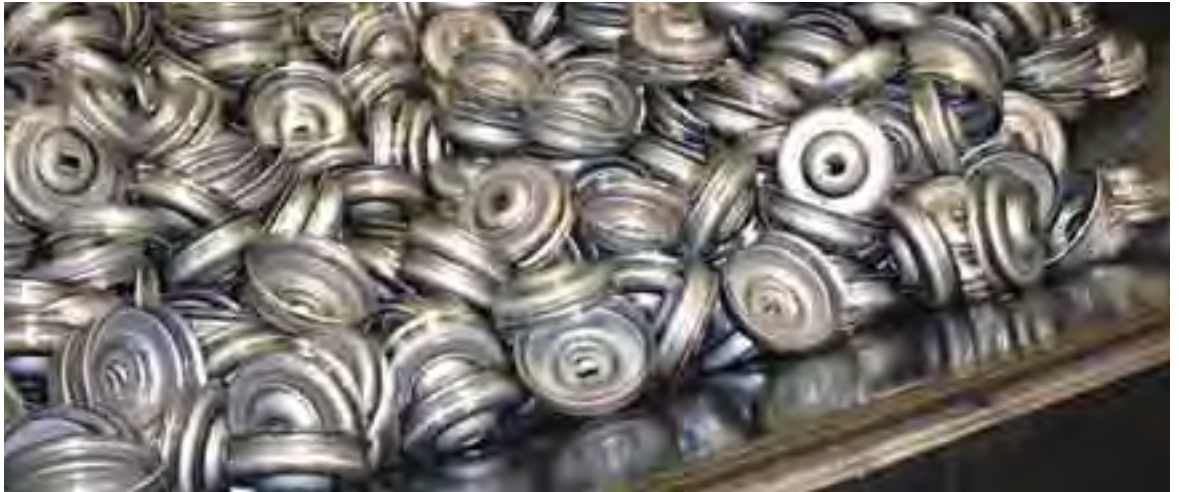
Like other parts produced from high-strength steels, these high-strength low-alloy steel seat spring brackets, stamped at Batesville Tool & Die, Batesville, IN, demand enhanced lubricant properties.
