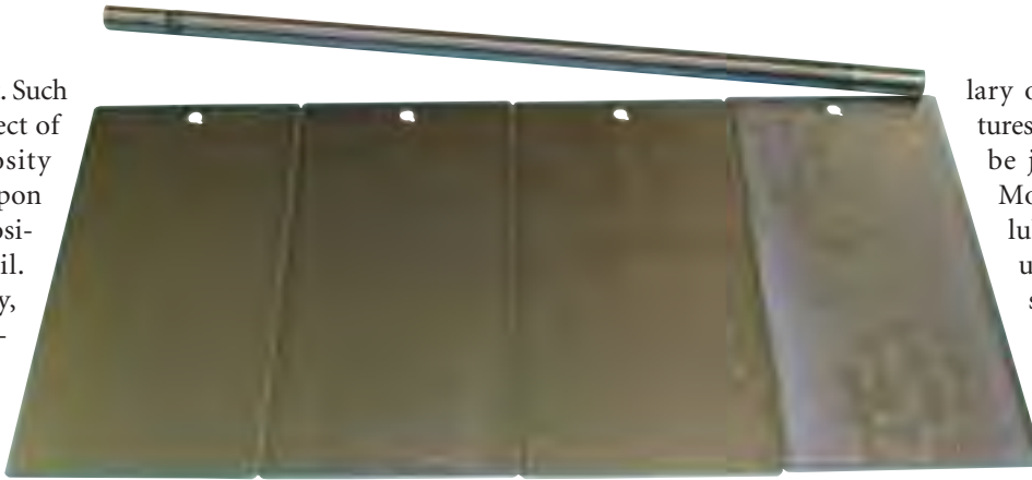
These high-strength-steel panels show the sheeting action of various lubricants. The first two, from left, show good and medium sheeting action respectively, from two different advanced technology synthetic lubricants; the third, a standard synthetic lubricant—poor sheeting; and the fourth, a standard emulsifiable chlorinated oil—poor sheeting.
